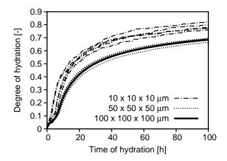
**FIGURE 3.** Effect of RVE sizes on degree of hydration, each with five random realizations
