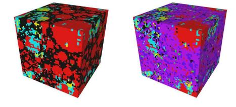
**FIGURE 1.** RVE  $50 \times 50 \times 50 \mu m$ , w/c = 0.25, initial (left) and at the degree of hydration of 0.63 (right). Dominant phases include water-filled porosity (black), C<sub>3</sub>S (red), C<sub>2</sub>S, C<sub>3</sub>A, C<sub>4</sub>AF, gypsum, CH (blue), and C-S-H (violet)
