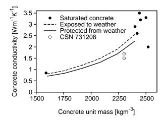
**FIGURE 5.** Thermal conductivity of mature concrete according to a Czech standard and [1]
