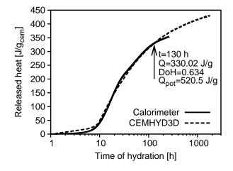
**FIGURE 7.** Isothermal calorimetry and CEMHYD3D simulation at  $25^{\circ}$ C, w/c = 0.5
