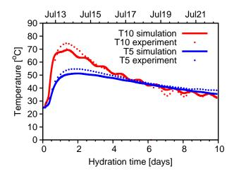
FIGURE 17. Temperature evolution in gauges T5 and T10
