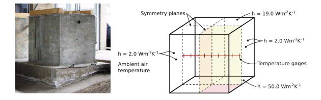
FIGURE 8. Experimental setup of a temperature measurement and corresponding quarter model (photo J. Litoš)
