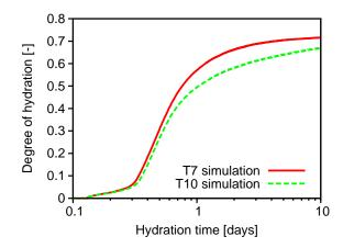
FIGURE 19. Evolution of hydration degree in gauges T7 and T10
