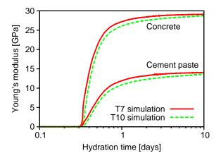
**FIGURE 20.** Predicted evolution of Young's modulus in gauges T7 and T10 on the scale of cement paste and concrete, no experimental data
