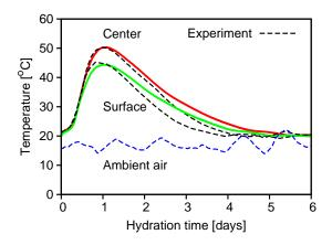
**FIGURE 9.** Validated heat evolution in the  $1 \times 1 \times 1$  m specimen
