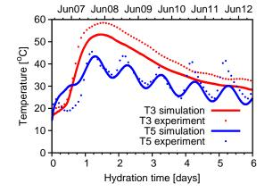
**FIGURE 13.** Temperature evolution in gauges T3 and T5
