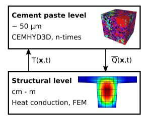
**FIGURE 4.** Coupling between the level of cement paste and structure
