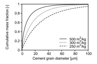
**FIGURE 2.** Assumed Rosin-Rammler cumulative distribution for cements with three Blaine finenesses according to Eqs. (1)–(3)
