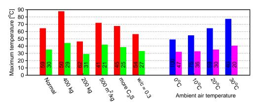
**FIGURE 22.** Maximum temperatures in the beam (left columns) and slab (right columns) when varying individual parameters of cement, concrete, or air temperature. Number in the bar represents time in hours when maximum temperature was reached
