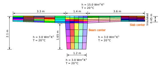
FIGURE 21. Topology of bridge cross section with the mesh, boundary conditions, and important node positions
