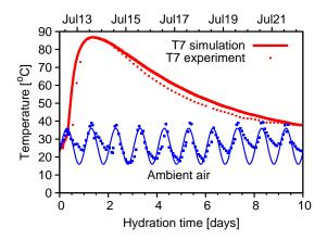
**FIGURE 16.** Temperature of central gauge T7 and approximated ambient air
