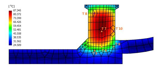
FIGURE 18. Temperature field at 1.367 days when the maximum in T7 is achieved
