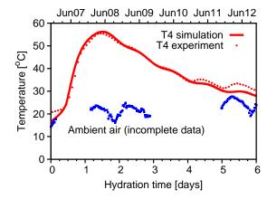
**FIGURE 12.** Temperature of central gauge T4 and ambient air temperature
