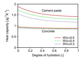
**FIGURE 6.** Heat capacity for cement paste and concrete predicted by the law of mixture
